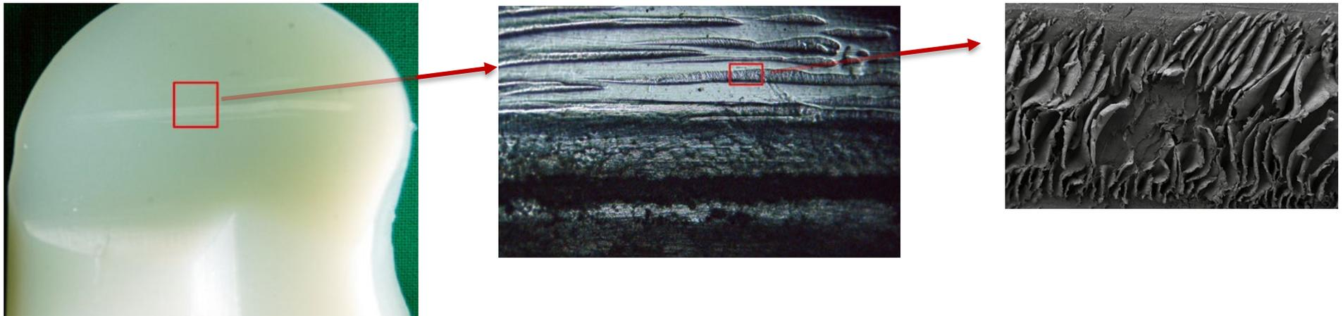
Most common form of backside wear
